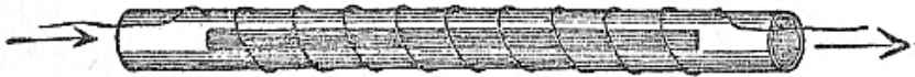
This is a picture of one of the needles that Savary probably used for his experiments with the helix. A very fine needle is wrapped around by a conducting wire, and its polarity is checked using a compass. In this picture, the needle is enclosed in a glass tube for insulation.
